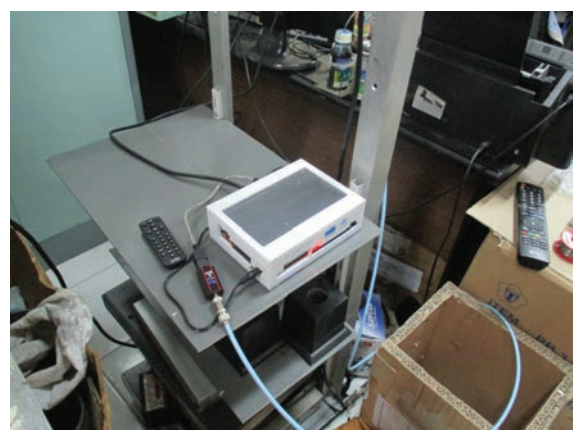
Gambar 11 Development Board A10 dan Demodulator + Tuner PCTV Nano Stick T2 (STB)
